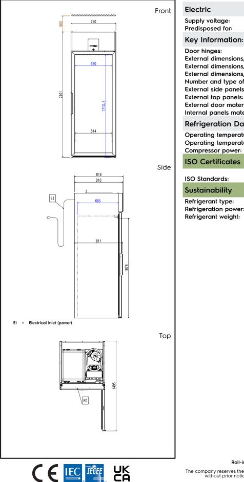
External dimensions, Width: 750 mm External dimensions, Depth: 810 mm External dimensions, Height: 2100 mm Number and type of doors: 1 Glass External side panels: 304 AISI External top panels: Galvanized Steel External door material: Glass 304 AISI Internal panels material: **Refrigeration Data** Operating temperature min.: 2 °C Operating temperature max.: 10 °C Compressor power: 1/3 hp **ISO Certificates** ISO 9001; ISO 14001; ISO **ISO Standards:** 45001; ISO 50001 Sustainability
